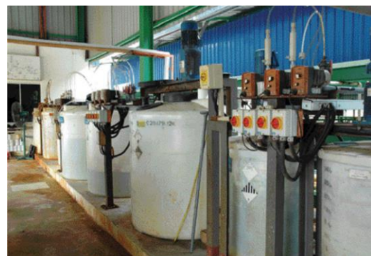
Figure 11.8: Physical treatment to detoxify the waste before final disposal to secured landfill
