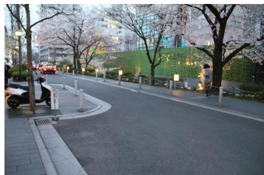
Figure 8.27: The use of chicanes in Kyoto to reduce vehicles speed (Source: Muhammad Zaly Shah)
